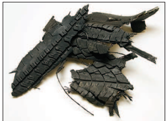
2" Shred Size with Steel Wire Still Present
